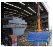
A key milestone was passed on the build of HMS Prince of Wales when the two 160 tonne diesel generators arrived at the shipyard.
