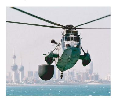
WESTLAND SEA KING ASaCS Mk 7 Primary Role Airborne Surveillance and Control Max Speed 120 Knots Crew 1x Pilot, 2x Observer Max Takeoff Weight 9,800kg Endurance 4 Hours Weapons Searchwater 2000 Radar
